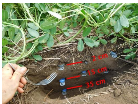
Figure 32 Installation des loggers
